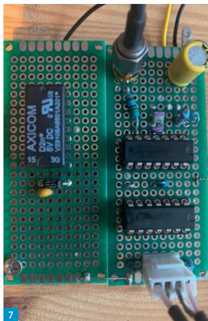
Fig. 5: Schematic of VCO. Fig. 6: Limiting the range of the VCO. Fig. 7: Top view of the VCO with relay for capacitor switching. Fig. 8: Alternative connection for a frequency counter.
